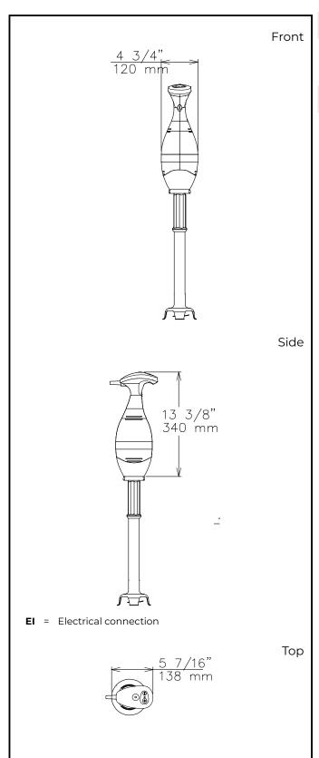
Electric Supply voltage: 110-120 V/1 ph/50/60 Hz **Total Watts:** 0.45 kW Plug type: USA NEMA 5-15P Key Information: External dimensions, Width: 5 7/16" (138 mm) External dimensions, 4 3/4" (120 mm) Depth: External dimensions, 30 1/8" (765 mm) Height: **Shipping width:** 11 7/16" (290 mm) Shipping depth: 27 3/16" (690 mm) Shipping height: 7 1/16" (180 mm) **Shipping weight:** 12 lbs (5.26 kg)
